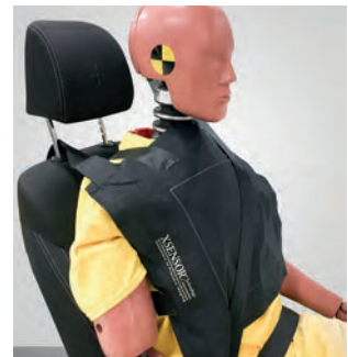
ABOVE LEFT: Custom vest equipped with XSensor technology ABOVE: A crash dummy wearing a vest ready for a seatbelt test
